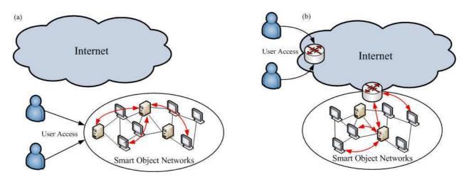
Fig. 1. Connectivity models: (a) autonomous smart object networks. (b) ubiquitous smart object networks.
