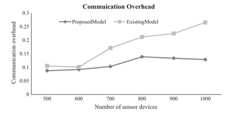
Fig. 5 Communication overhead considering total node death for varied sensor devices.
