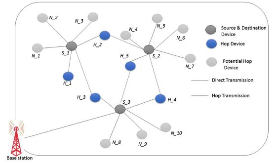
Fig. 1 Architecture of proposed energy efficient Hop selection model for sensor network.
