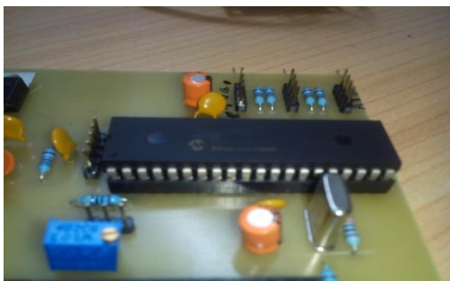
Fig.3 PIC microcontroller PIC18F45K22
