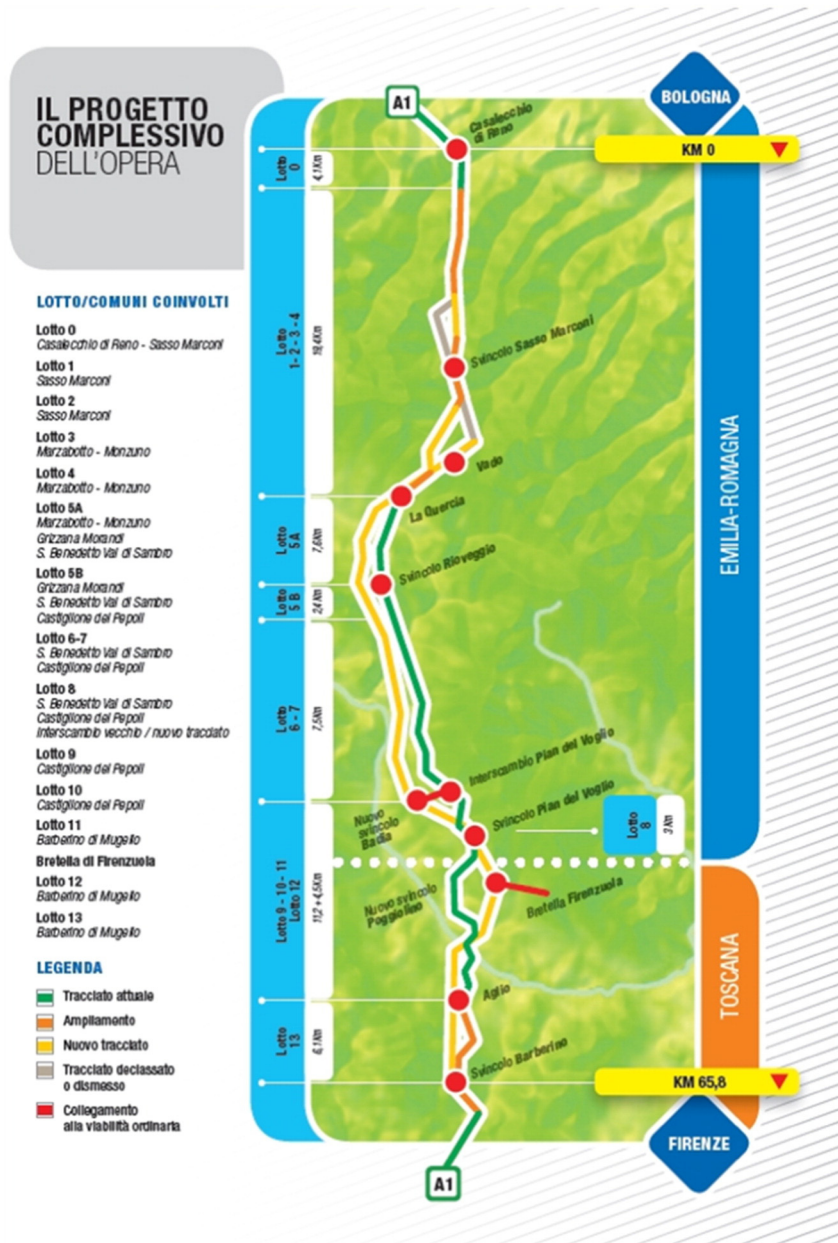
Fig. 1. The Variante di Valico Megaproject . This figure shows the overall layout of the Variante di Valico. It highlights the different lots which compose the megaproject and the various territories which are affected by it. The green line represents the current route; the orange line is the upgrade and enlargement of the current route; the yellow line is the new route; the grey line is the downgraded or abandoned route and the red dots represent the connection to the ordinary roads.
