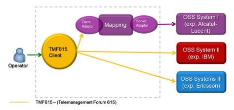
Fig. 5 Proposed OSS architecture
