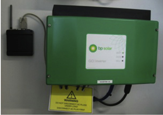
Fig. 2. Example of a VPS node, consisting of a SMA inverter connected to an embedded controller with wifi communications.
