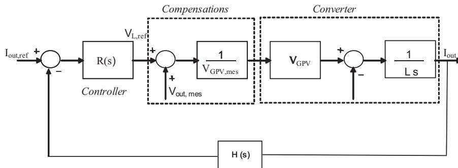
Fig. 8. Control loop structure of alternative output current.
