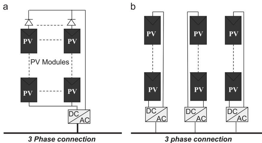
Fig. 3. (a) Centralized technology. (b) String technology.
