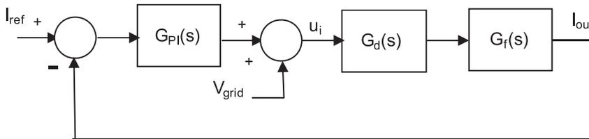
Fig. 13. Inverter current loop with PI controller.
