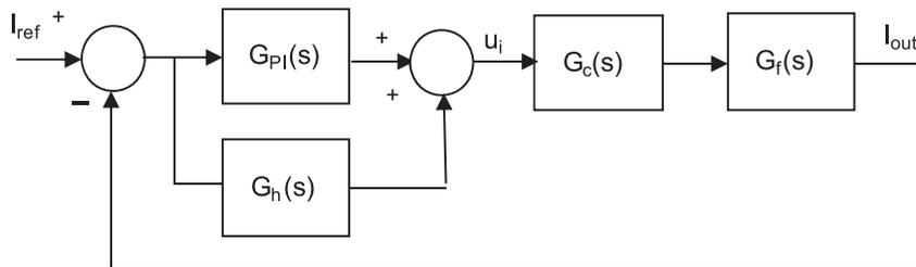
Fig. 14. Inverter current loop with PR controller.
