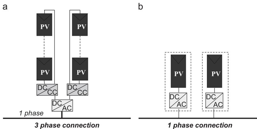
Fig. 4. (a) Multistring technology. (b) AC Module.
