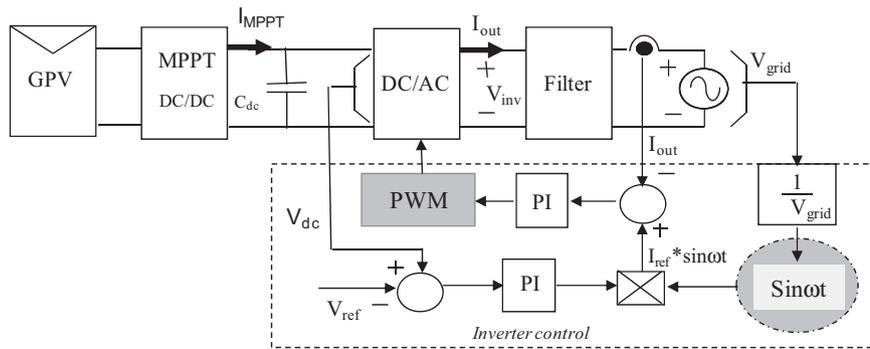
Fig. 7. Control structure with DC–DC converter and L Filter.
