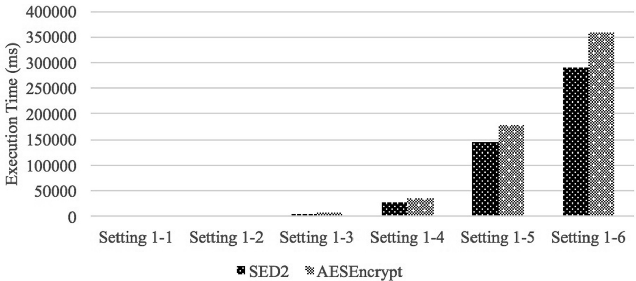
Fig. 8. Comparisons of the encryption execution time between SED2 (before document is sent out) and AES using settings 1-1, 1-2, 1-3, 1-4, 1-5, and 1-6.
