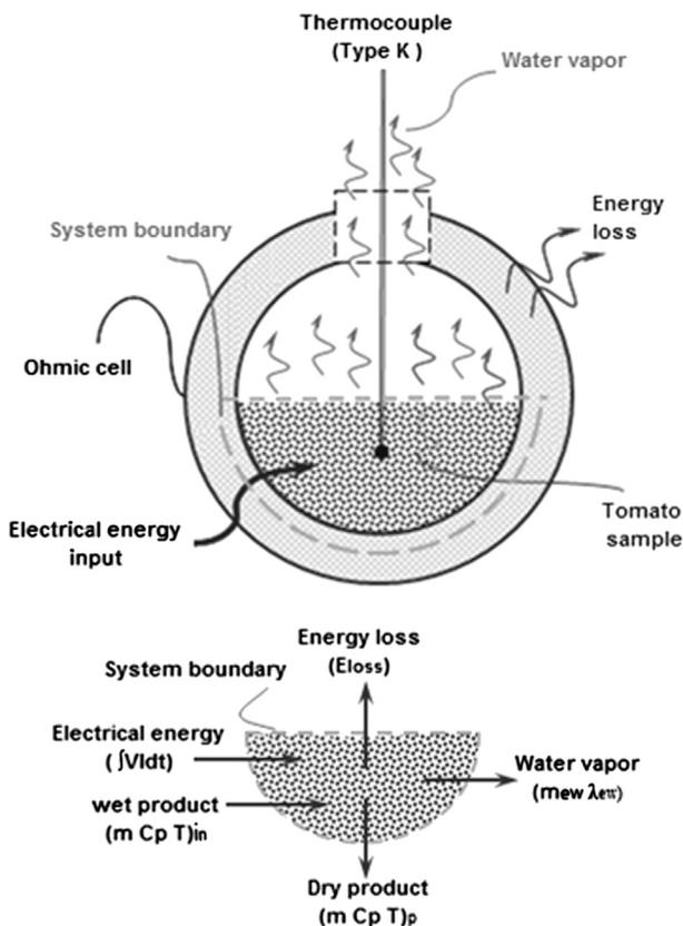
Fig. 2. Volume control of ohmic heating system.
