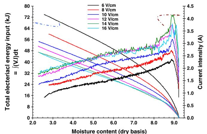
Fig. 8. Variation of electrical energy input and current intensity at different voltage gradients.
