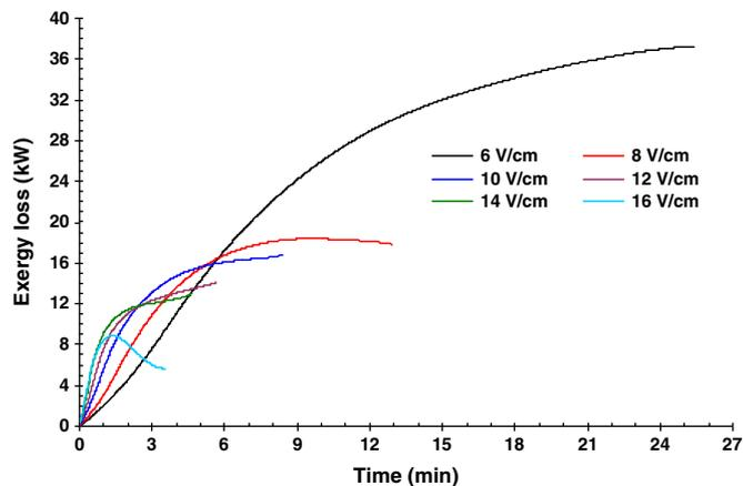
Fig. 11. Influence of voltage gradient on the exergy loss of tomato heating.
