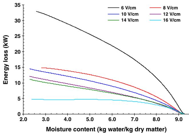
Fig. 6. Variation of energy loss with moisture content.
