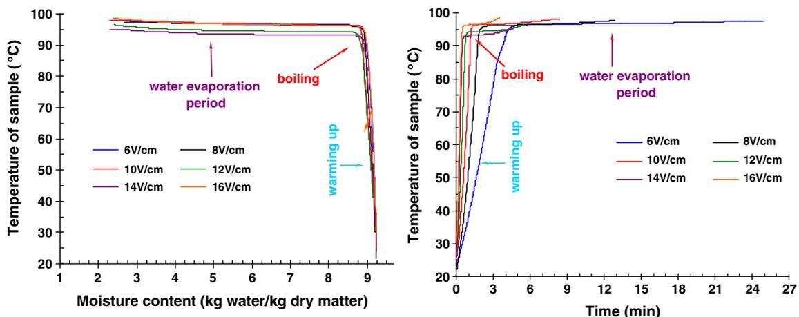
Fig. 4. Temperature of tomato samples during ohmic heating.
