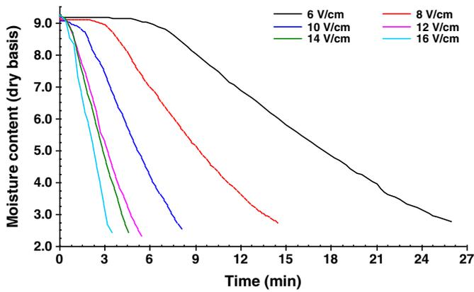
Fig. 3. Variations of moisture content as a function of time for different voltage gradient.
