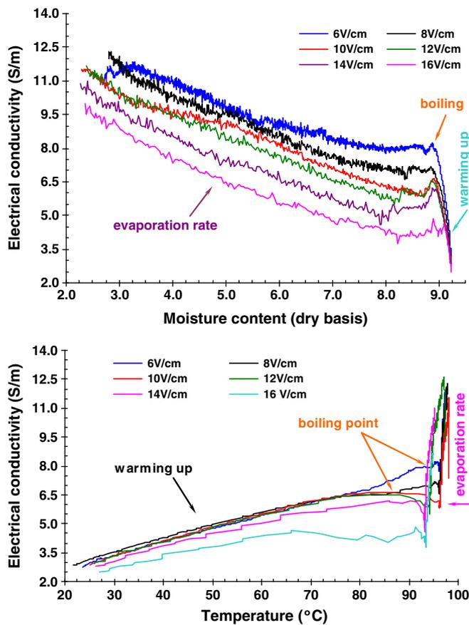
Fig. 9. Electrical conductivity changes of the tomato samples during ohmic heating.
