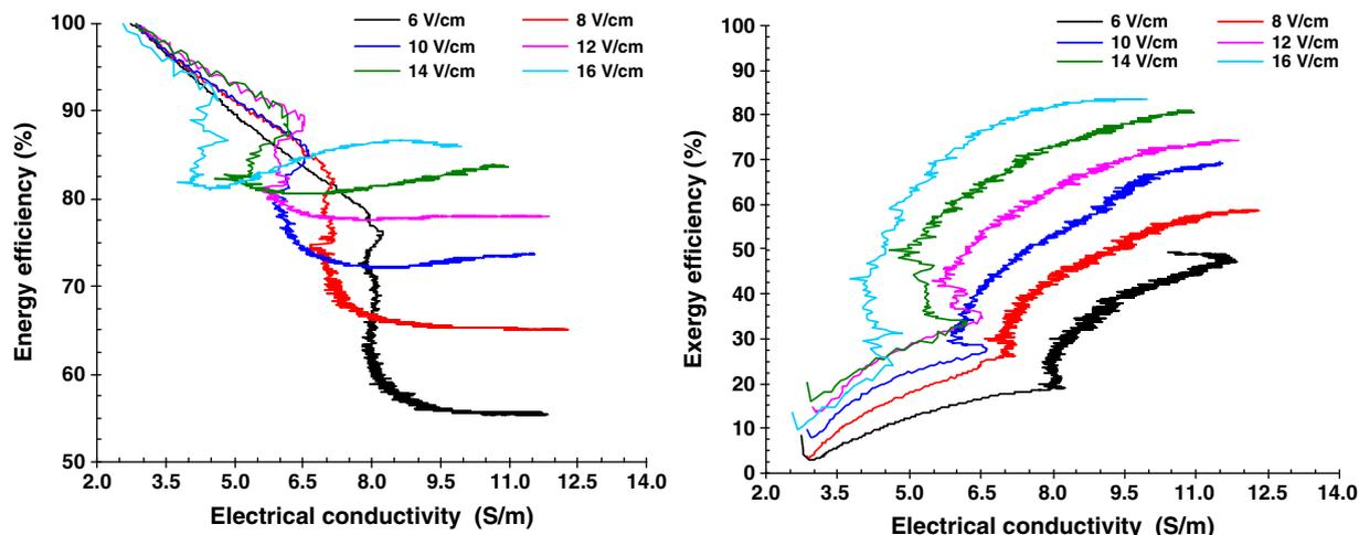
Fig. 12. Variations of energy and exergy efficiencies with electrical conductivity.
