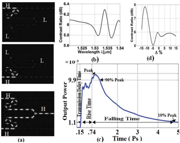
Fig. 9. Results of the proposed AND gate: (a) steady state field distribution, (b) contrast ratios, (c) time evolving curve of the output power, (d) fabrication tolerance.
