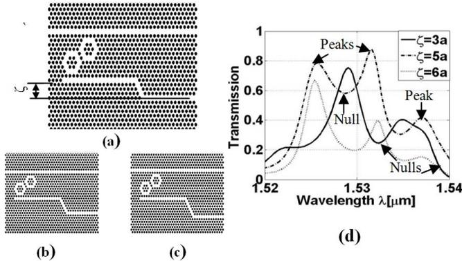
Fig. 8. Bend with different  $\zeta$ , (a)  $\zeta = 3a$ , (b)  $\zeta = 5a$ , (c)  $\zeta = 6a$ . (d) Transmission spectrum.
