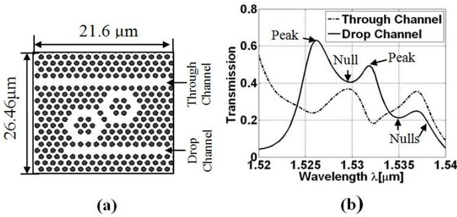
Fig. 7. Simulation of PhC resonator: (a) Structure. (b) Transmission.
