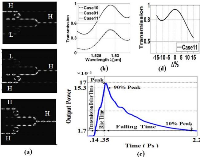
Fig. 5. Results of the proposed OR gate: (a) steady state field distribution, (b) transmission spectrum, (c) time evolving curve of the output power, (d) fabrication tolerance.
