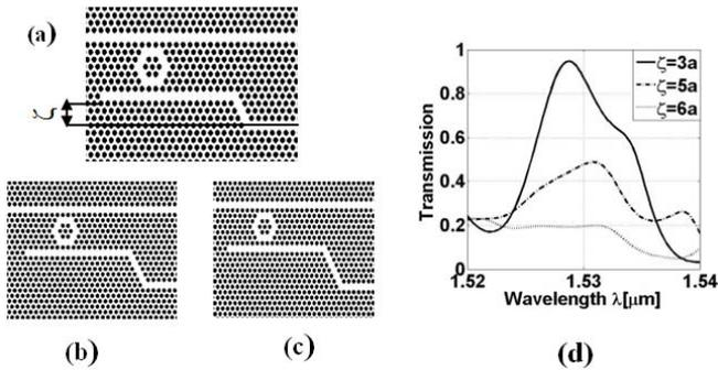
Fig. 4. Bend with different  $\zeta$ , (a)  $\zeta = 3a$ , (b)  $\zeta = 5a$ , (c)  $\zeta = 6a$ . (d) Transmission.
