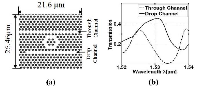
Fig. 3. Simulation of ring cavity: (a) Structure. (b) Transmission.
