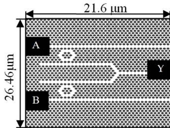
Fig. 2. The proposed optical OR gate structure.
