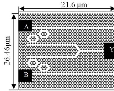
Fig. 6. The proposed optical AND gate structure.
