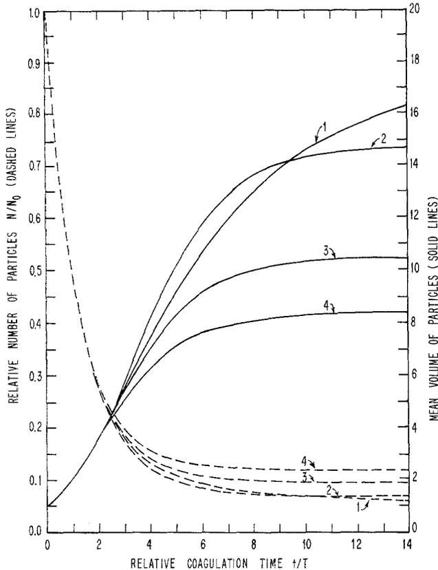
FIG. 2. Effect of conjunction and breakup on floe growth and total number of particles in orthokinetic coagulation.  $C = 0.01$ ,  $MAXVOL = 20$ ,  $T = 17.7$ ; 1, BRAKUP 1 (Run 21); 2, BRAKUP 2 (Run 29); 3, BRAKUP 3 (Run 13); 4, BRAKUP 4 (Run 30).
