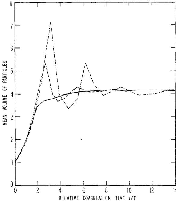
FIG. 4. Effect of input variables on floc growth in orthokinetic coagulation. MAXVOL = 20, BRAKUP = 10; Run 45,  $C = 0.04$ ,  $T = 4.09$  —; Run 46,  $C = 0.08$ ,  $T = 1.84$ , ----; Run 47,  $C = 0.10$ ,  $T = 1.42$  -.-.-.
