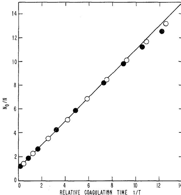
FIG. 1. Linearizing plot for second-order decrease in total number of particles in perikinetic coagulation.  $\circ$  Run 24,  $\bullet$  Run 26, analytic solution by Smoluchowski shown as solid line.
