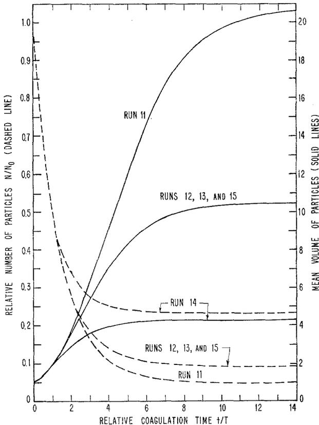
FIG. 3. Effect of other input variables on flocculation and total number of particles in orthokinetic coagulation. All runs used BRAKUP 3. Run 11,  $C = 0.02$ ,  $MAXVOL = 40$ ,  $T = 8.7$ ; Run 12,  $C = 0.04$ ,  $MAXVOL = 20$ ,  $T = 4.0$ ; Run 13,  $C = 0.01$ ,  $MAXVOL = 20$ ,  $T = 17.7$ ; Run 14,  $C = 0.01$ ,  $MAXVOL = 8$ ,  $T = 18.6$ ; Run 15,  $C = 0.02$ ,  $MAXVOL = 20$ ,  $T = 8.7$ .
