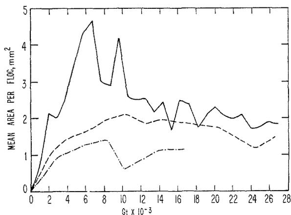
FIG. 5. Variation in mean floc size during flocculation.  $\text{Fe}_2(\text{SO}_4)_3 = 1.6 \times 10^{-4}$  mole/liter,  $\text{NaHCO}_3 = 1 \times 10^{-2}$  mole/liter,  $G$  = Mean Shear Gradient ( $\text{sec}^{-1}$ ),  $t$  = time of flocculation ( $\text{sec}.$ ),  $\text{pH} = 6.8$ ; —  $G = 3.2$ ; ----  $G = 6.8$ ; -·-·-  $G = 9.3$ .
