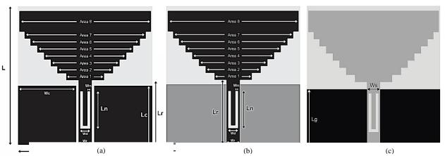
Fig. 1. (a) CPW-fed antenna (front) (b) MS-fed antenna (front) (c) MS-fed antenna (back)
