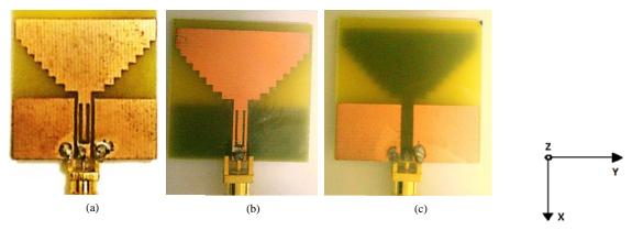
Fig. 2. Prototype (a) CPW-fed antenna (front) (b) MS-fed antenna (front) (c) MS-fed antenna (back)
