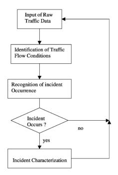
Fig. 1. Architecture of the proposed fuzzy clustering-based algorithm.
