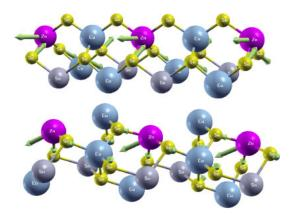
**Fig. 2.** (Color online) Snapshots of the hardest transversal optical mode in KS ( $239 \text{ cm}^{-1}$ , top image) and ST ( $254 \text{ cm}^{-1}$ , bottom image) phases of CZTSe. Arrows indicate relative displacement of ions, as follows from phonon mode eigenvectors.
