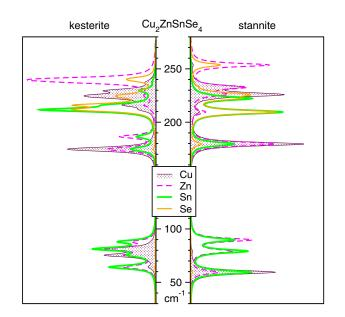
**Fig. 1.** (Color online) Density of zone-center vibration modes, resolved in atomic contributions, for KS and ST-type CZTSe. For convenience, discrete peaks are artificially broadened with halfwidth parameter  $2 \text{ cm}^{-1}$ . The magnitudes of peaks are in arbitrary, but identical, units, attributed to one atom of each type.
