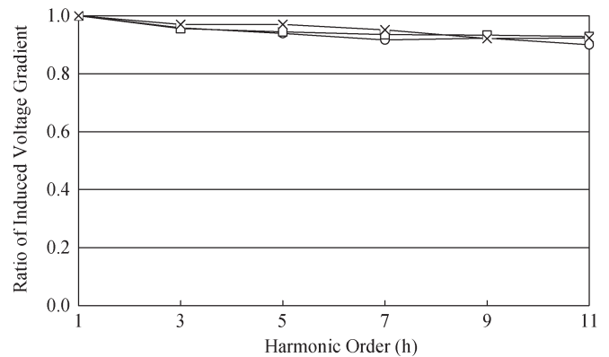
Fig. 4. Induced armor voltages for the cables in free air. □ FS configuration. ○ FT configuration. × TF configuration.
