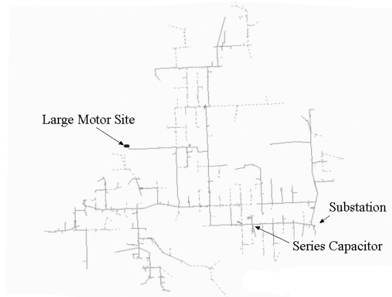
Fig. 6. Motor start with the series capacitor in service, only a small section of the feeder has voltage fluctuations above 5%.
