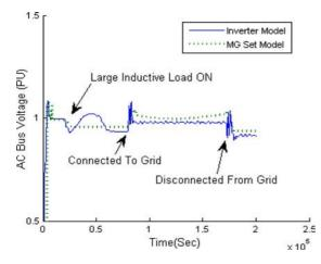
Fig. 23. Variation in the supply voltage in sudden grid connected and isolated modes.
