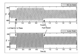
Fig. 25. Comparison of Voltage Swell of un-faulted phase for both generic and retrofitted HPS systems.
