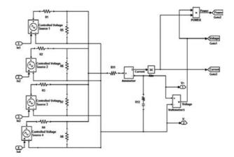
Fig. 7. MATLAB/Simulink model of the dc bus.
