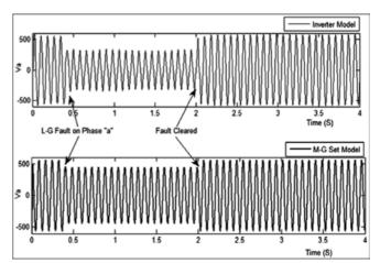
Fig. 24. Comparison of Voltage Sag of faulted phase for both generic and retrofitted HPS systems.
