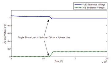
Fig. 26. Positive and Negative Sequence voltages of Inverter based generic HPS.
