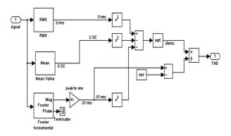
Fig. 16. Matlab/Simulink Modeling of THD block.
