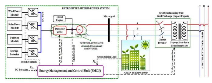
Fig. 4. The architecture of the retrofitted HPS connected to the building and running in parallel with utility grid.
