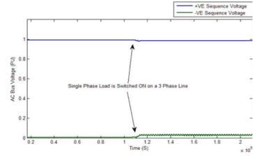
Fig. 27. Positive and Negative Sequence voltages of MG set based retrofitted HPS.
