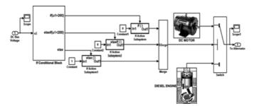
Fig. 12. MATLAB/Simulink model for switching between dc Motor and Diesel engine to drive alternator.
