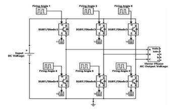
Fig. 8. MATLAB/Simulink model of Inverter.
