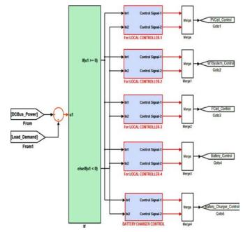
Fig. 15. MATLAB/Simulink model of EMCU.
