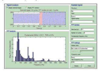
Fig. 18. THD analysis for retrofitted HPS architecture.
