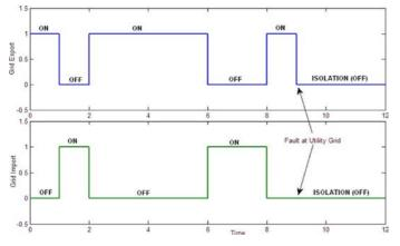
Fig. 36. EMCU Control signals to grid synchronizing unit for grid import/export/isolate.
