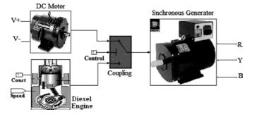
Fig. 10. MATLAB/Simulink model of dc motor/Diesel engine-Synchronous generator set.
