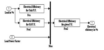
Fig. 19. Matlab/Simulink Model for electrical efficiency.
