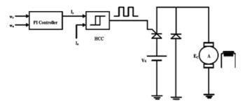
Fig. 11. Speed controller circuit for dc Motor.
