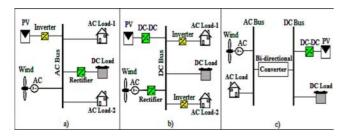
Fig. 1. Different architectures of standalone HPS.
