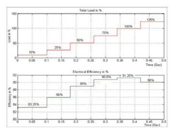
Fig. 20. Electrical Efficiency at different loads for retrofitted HPS architecture.
