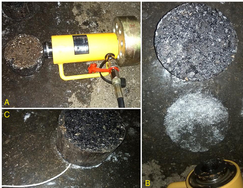
Fig. 7. Scene pictures for testing the horizontal ice adhesive force (A. quasi-static loading; B. specimen bottom and ice marks after test; C. ice temperature measurement).
