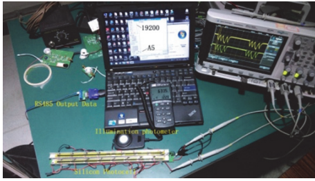
FIGURE 10: Energy gathering and signal detecting demo system.
