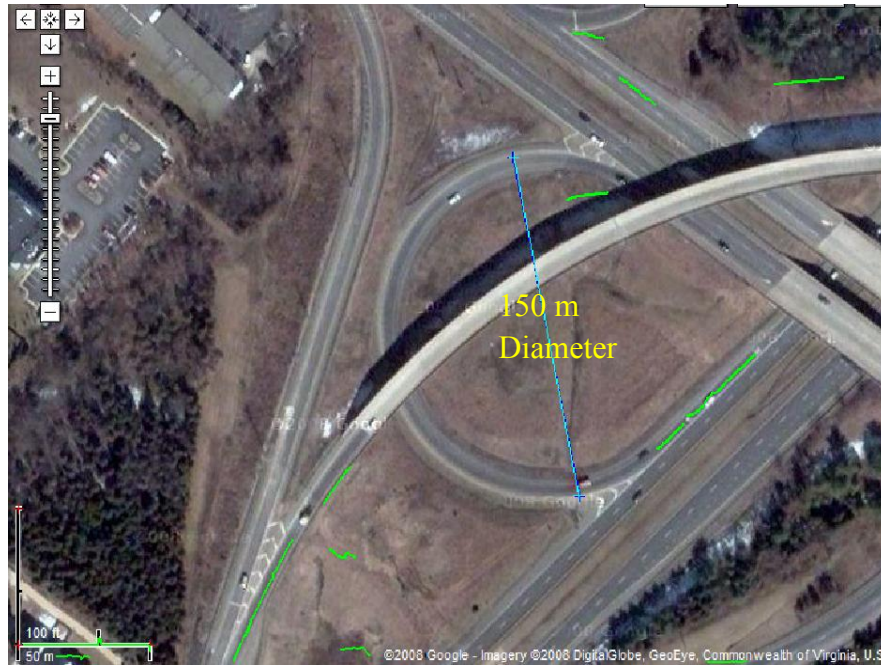
Figure 1 – Typical Tight Radius Freeway Interchange Ramp Design (75 meters)
