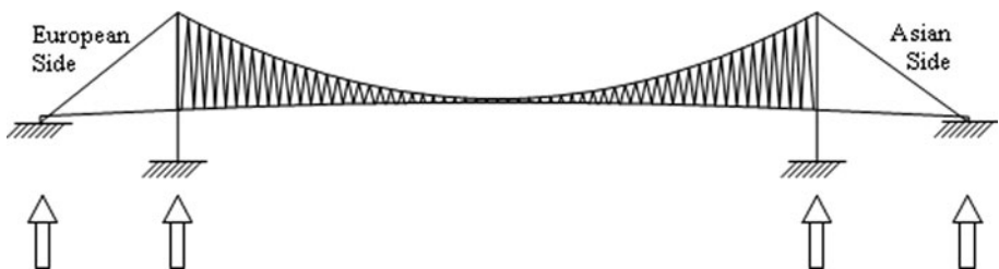
Fig. 6 2D finite element model of Boğaziçi (First Bosphorus) suspension bridge subjected to vertical ground motions
