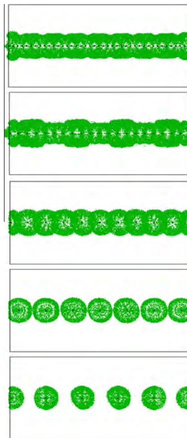
Fig. 5. Illustration of stress wave front at 0.2 ms ( S : Spacing).
