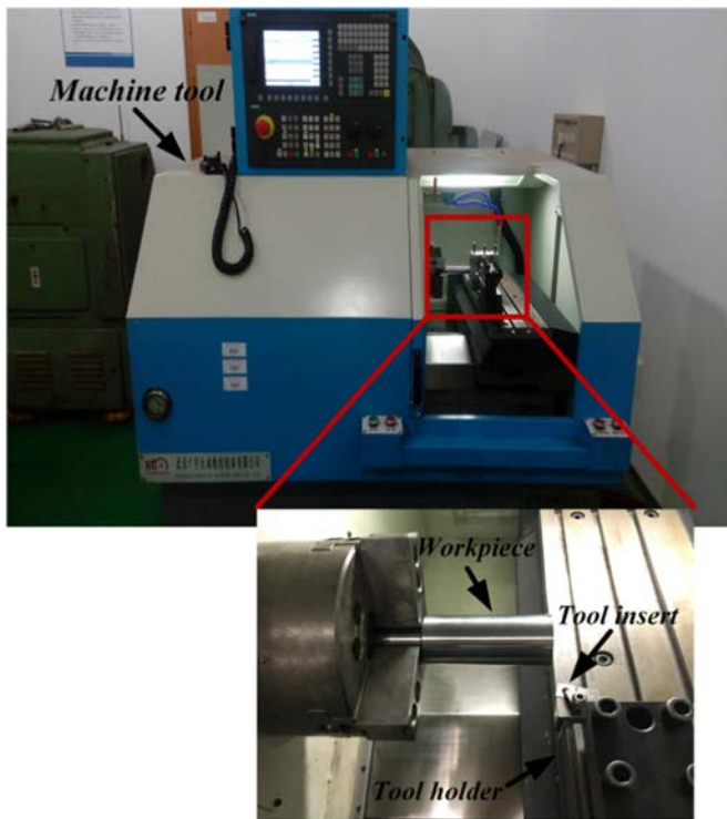
Fig. 5. Experimental set-up for the turning tests.
