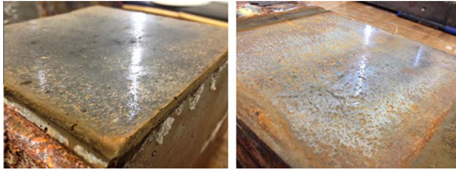
Fig. 5. Post-test grout (left) and steel (right) surfaces of a wet sample.
