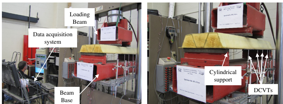
Fig. 9. Four-point bending flexural test setup.
