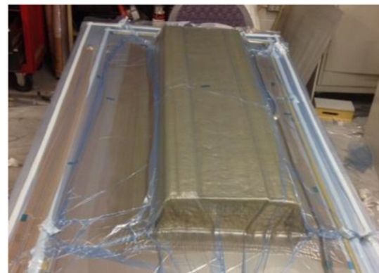
Fig. 7. VARTM manufacturing process for mid-scale panels.
