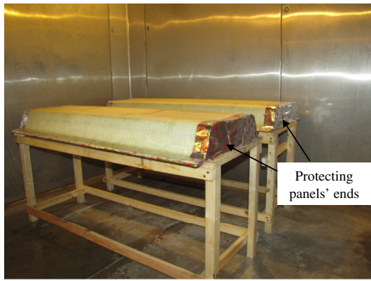
Fig. 8. PU sandwich panels within environmental test chamber.
