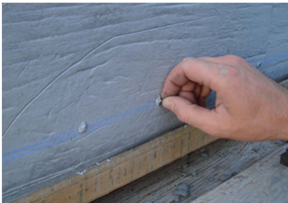
Fig. 2. Placement of DEMEC points.
