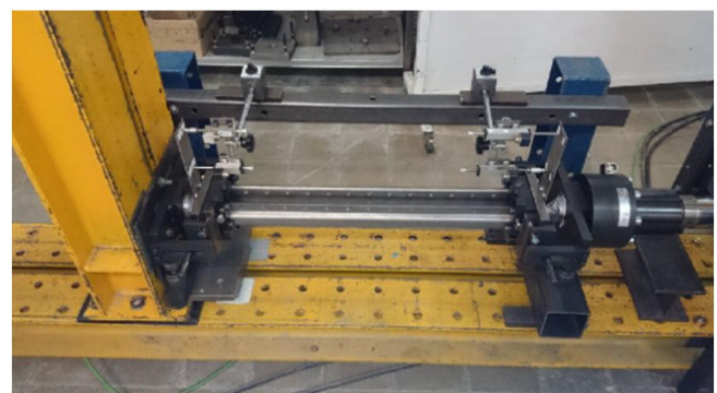
Fig. 8. Set-up of the displacement transducers used to obtain the axial displacement of the rack upright.
