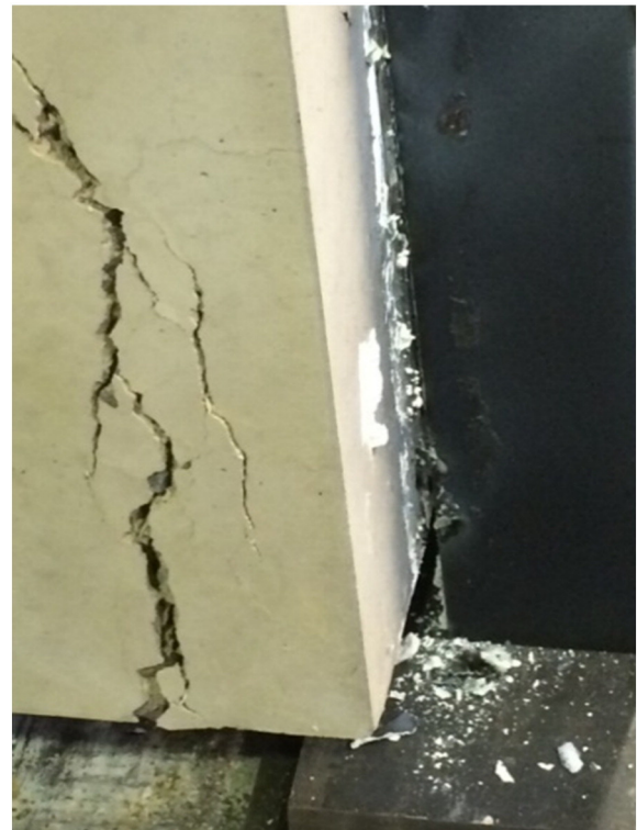
Fig. 6. Failure mode of headed stud shear connector specimens post-fire.
