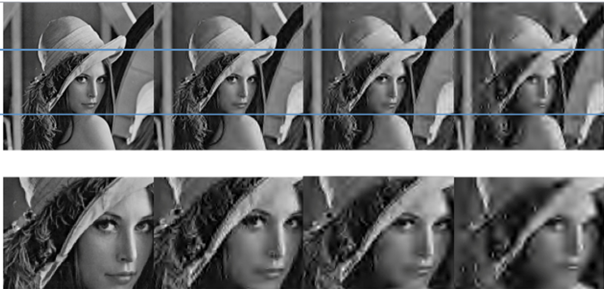
Fig. 2 With EZW compression, from left to right, under different levels of communication channel noise.
