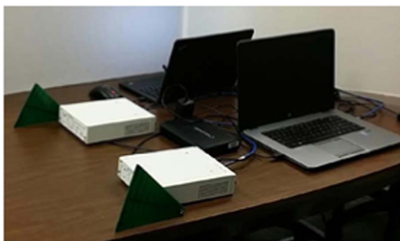
Fig. 5. System Experimental Setup with USRP, antenna and laptop.
