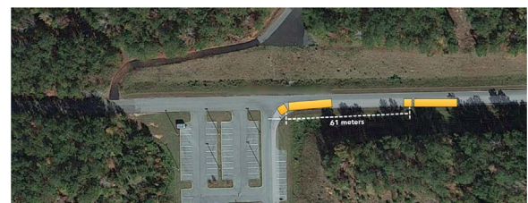
Fig. 6. Static test setup in Location B where the front truck is turning.
