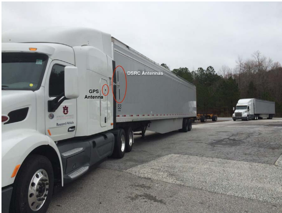
Fig. 3. Left side of a truck with one of the DSRC antennas and GPS antenna shown. The other DSRC antenna is mounted on the right side.
