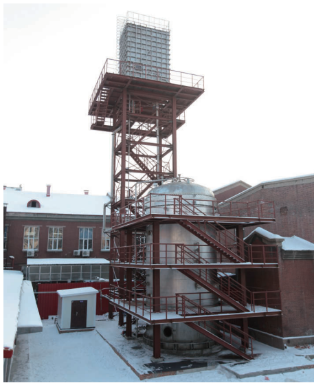
Fig. 8. Passive containment heat removal system (PCS) comprehensive performance test facility.
