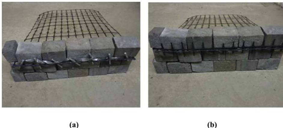
Fig. 8. Connection modes between geogrid and blocks: (a) mechanical connection; (b) frictional connection.
