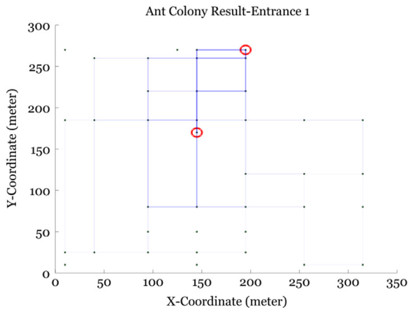
Fig. 4. Result of route finding for entrance 1 based on ant colony algorithms.
