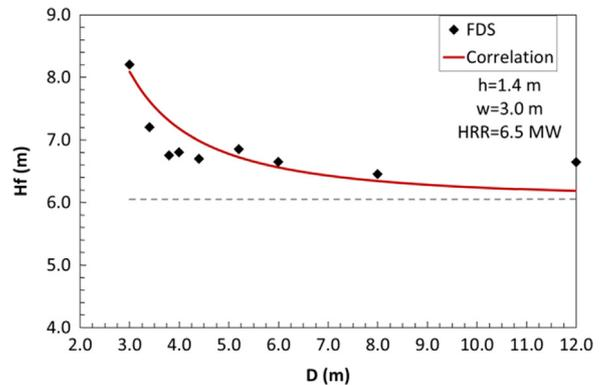
Fig. 12. Mean flame height vs. sidewall distances ( $D$ )  $h=1.4$  m;  $w=3.0$  m.
