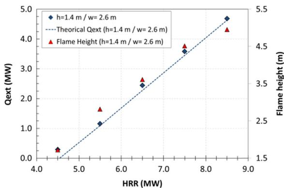
Fig. 8. Excess heat release rate and flame height as a function of the heat release rate.
