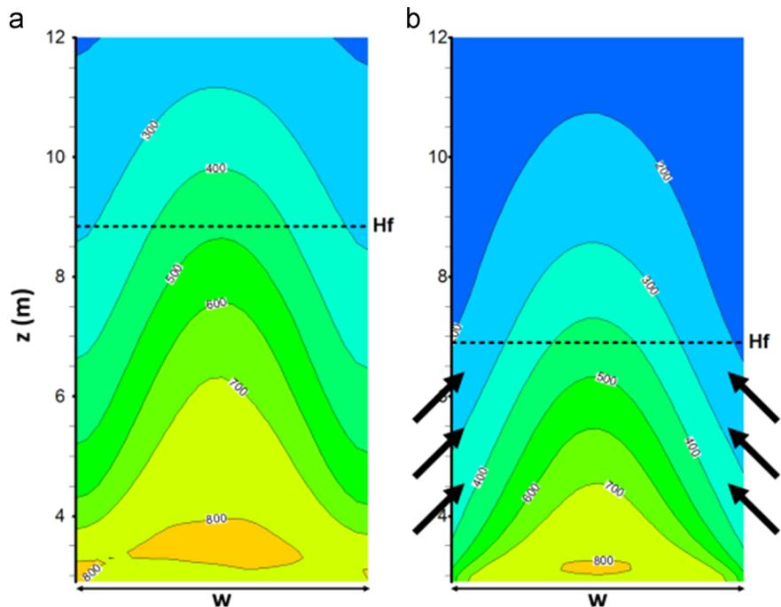
Fig. 14. Time-averaged wall temperature contours above the opening ( $h=1.4$  m;  $w=2.6$  m): a)  $D=2.6$  m; b)  $D=5.2$  m.
