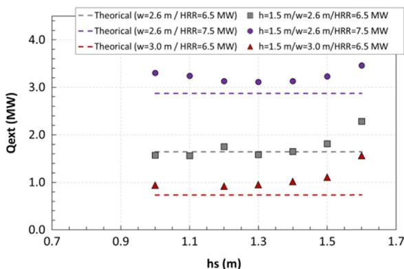
Fig. 7. Excess heat release as a function of the opening position "hs" (h = 1.5 m).
