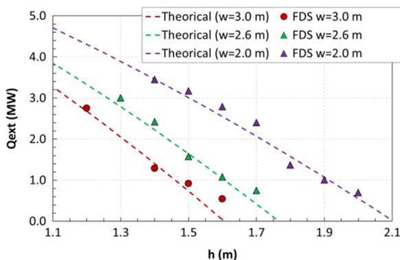
Fig. 6. Excess heat release as a function of the opening width "w".
