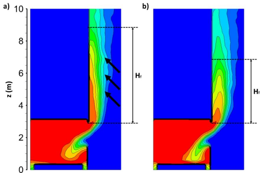
Fig. 13. Time-averaged temperature contours in the middle plane of the opening ( $h=1.4$  m;  $w=2.6$  m): a)  $D=2.6$  m; b)  $D=5.2$  m.
