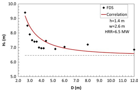
Fig. 10. Mean flame height vs. sidewall distances ( $D$ )  $h=1.4$  m;  $w=2.6$  m.
