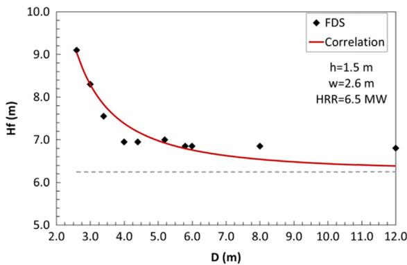
Fig. 11. Mean flame height vs. sidewall distances ( $D$ )  $h=1.5$  m;  $w=2.6$  m.
