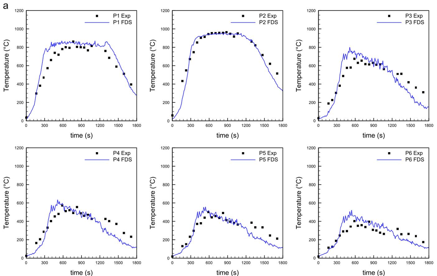
Fig. 3. (a) Temporal evolution of external temperatures at position P. (b) Temporal evolution of external temperatures at position Q. (c) Temporal evolution of external temperatures at position R.
