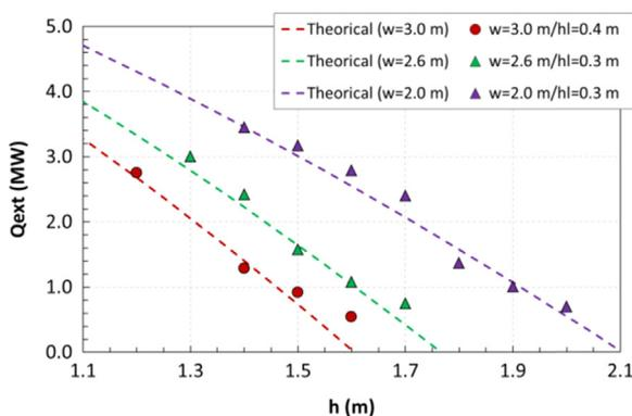
Fig. 5. Excess heat release as a function of opening height "h".
