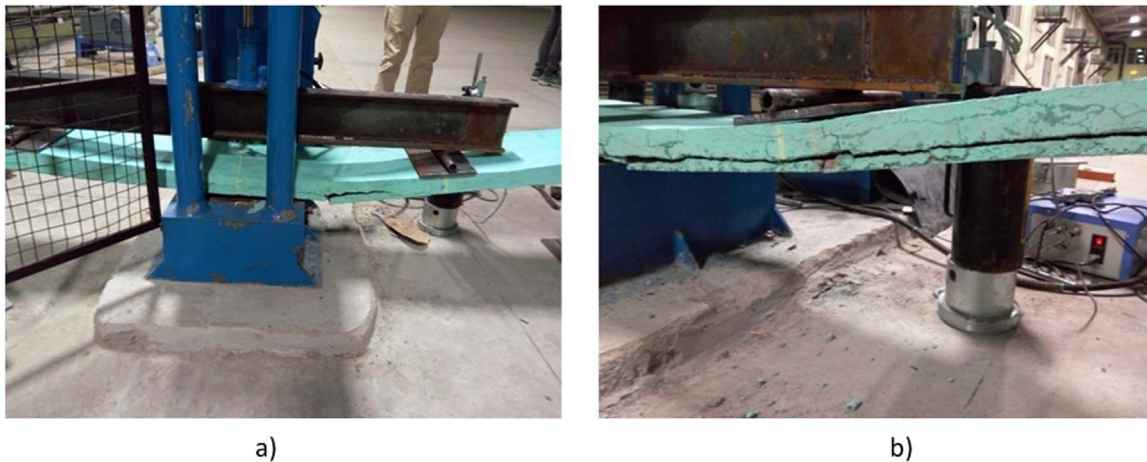
Fig. 8. a) Debonding failure, b) Closer view of debonding failure.
