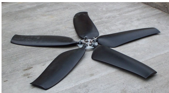
Fig. 6 A 1.618m Propeller fan wheel with 5 blades
