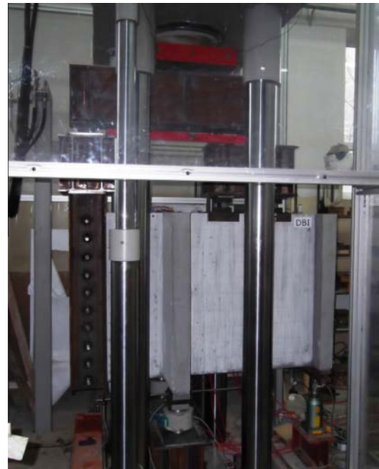
Fig. 9. Test set-up of DBI deep beams.
