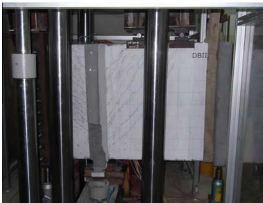
Fig. 19. Crack pattern of DBII deep beam after failure.
