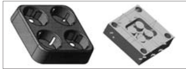
Figure 4 A 3D model of the multi socket body and the appropriate fixed mold plate
