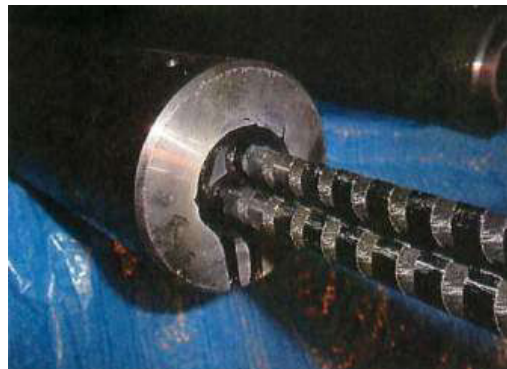
Figure 21. Steel sleeve with three CFRP rods
