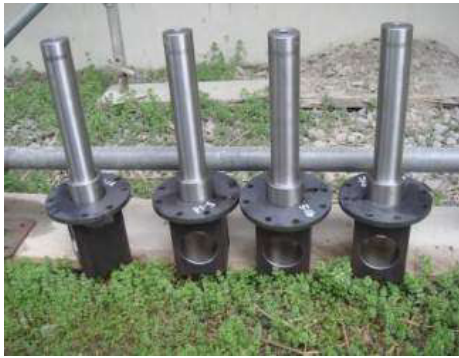
Figure 4. Anchors for ACM brace
