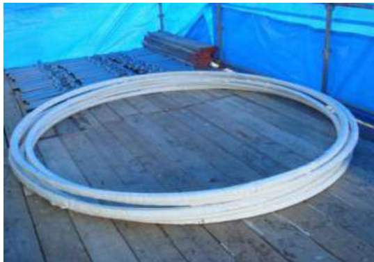
Figure 6. CFRP rod ( \phi 10\text{mm} , 5@100m)
