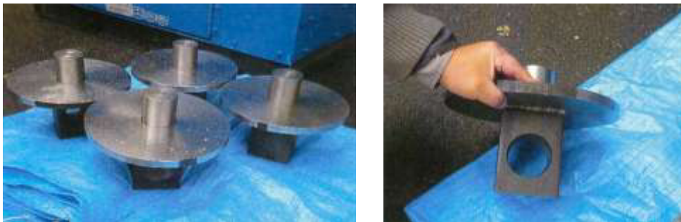
Figure 11. Anchors for ACM brace
