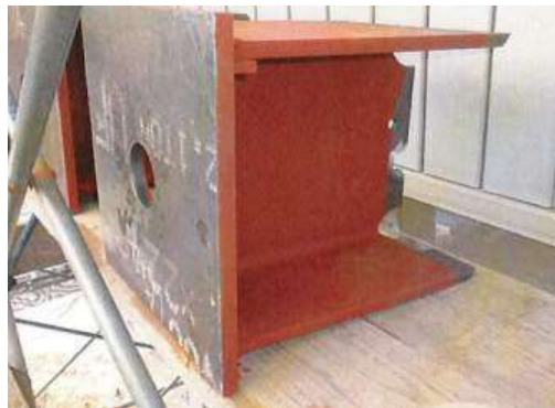
Figure 13. Steel bracket for ACM brace
