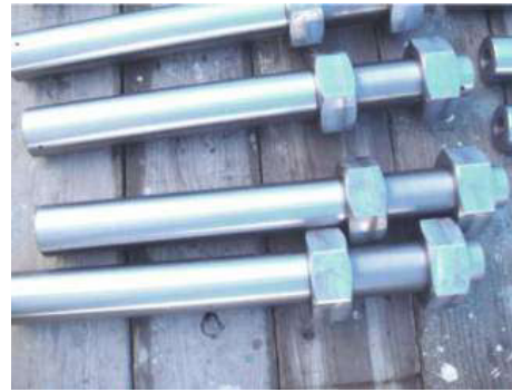
Figure 5. Steel sleeves for ACM brace
