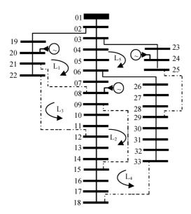
Fig. 3. 33-bus radial distribution system for  $HV^1$ .
