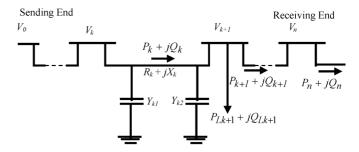
Fig. 1. Single-line diagram of a main feeder.
