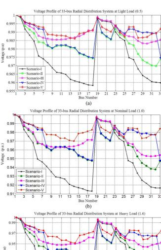
Fig. 7. Voltage profiles of 33-bus system at light, nominal, and heavy load conditions.
