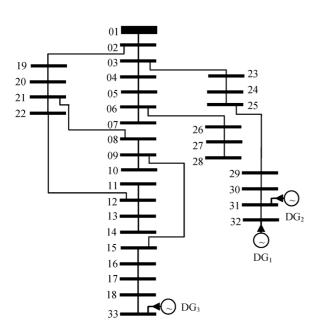
Fig. 6. Optimal network structure after simultaneous reconfiguration and DG installation.
