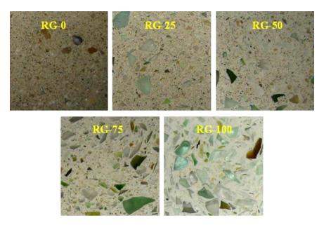
Fig. 5. Glass-architectural mortar featuring different replacement level of RG.
