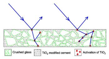
Fig. 4. Pathways of light and activation of  ${\rm TiO_2}$  in concrete block surface layer using glass as aggregates.
