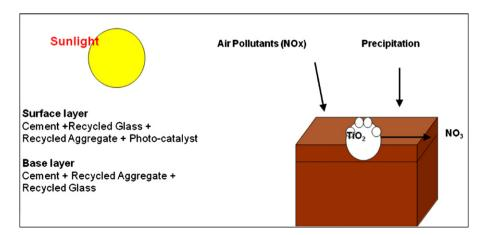
Fig. 3. Two-layer block structure prepared with different ingredients.
