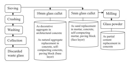
Fig. 1. Steps of converting waste glass to valuable materials and its applications.
