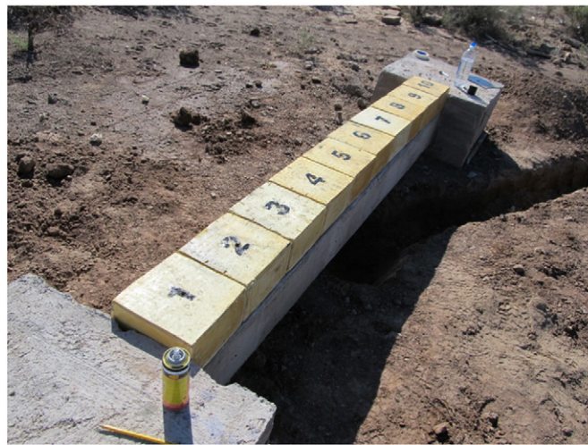
Fig. 8. Reinforced polyurethane bricks over the member.
