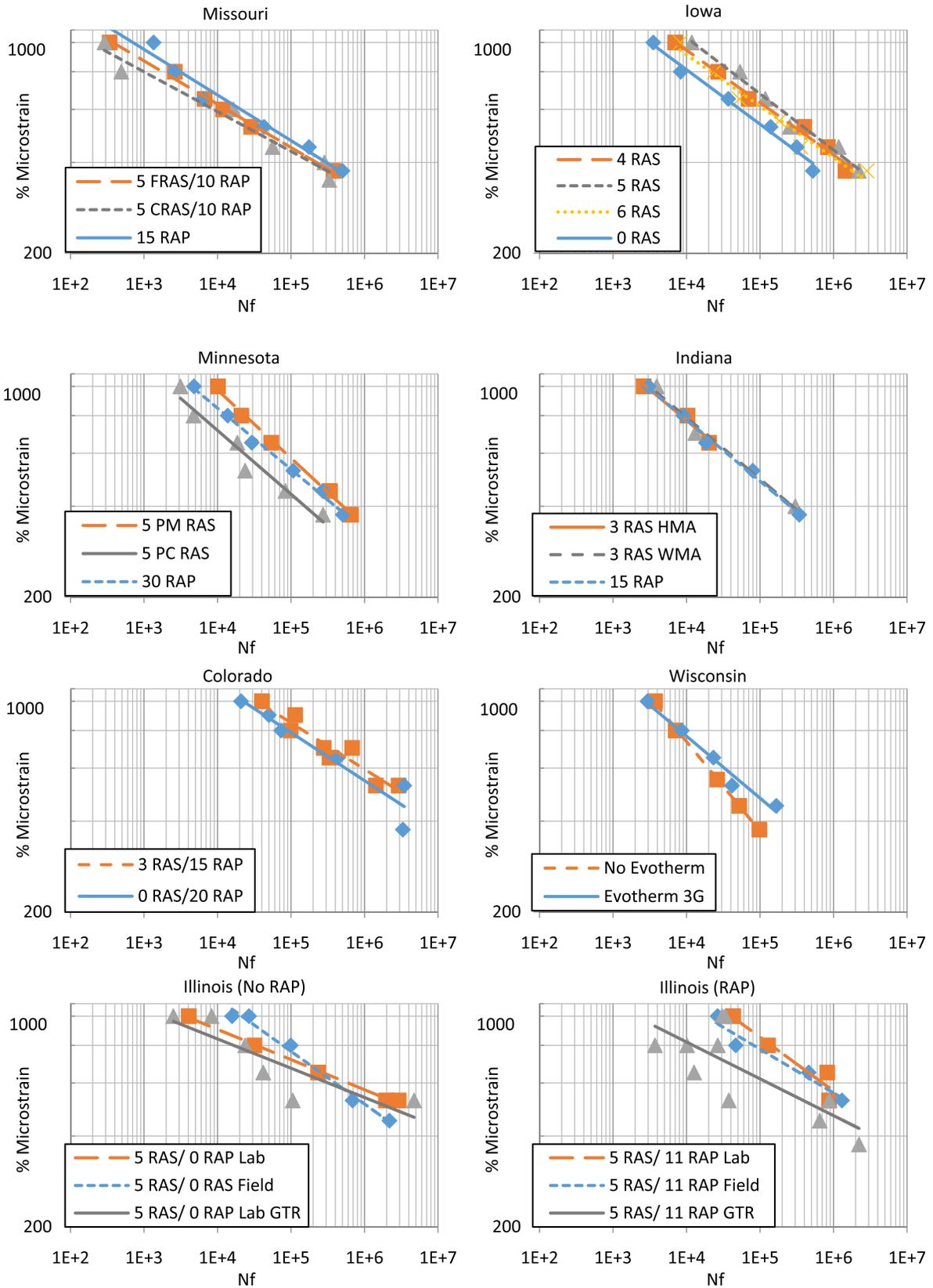
Fig. 8. Four-point bending beam fatigue curves.
