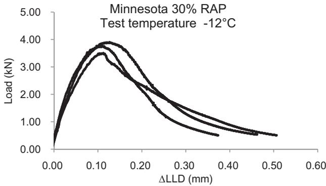
Fig. 2. Typical LLD versus load plot of three test replicates.
