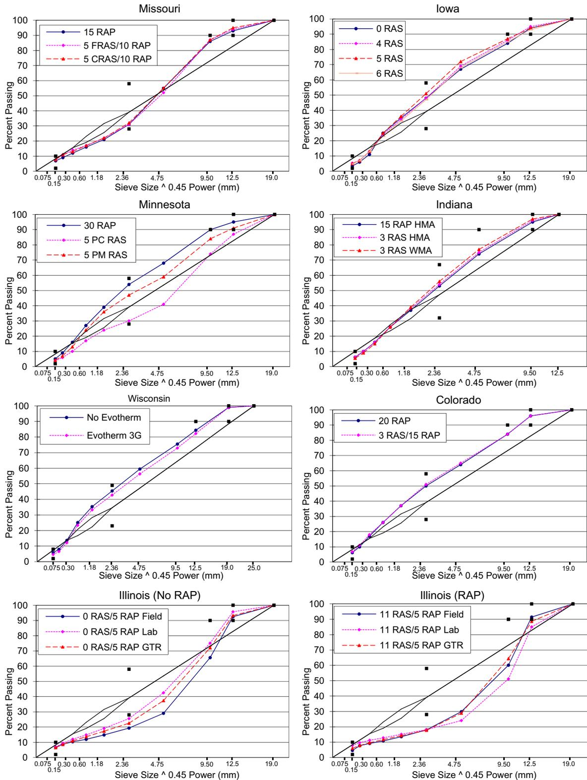
Fig. 5. Aggregate gradations.
