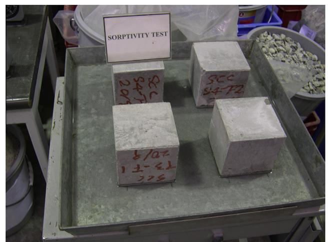
Fig. 2. Sorptivity test.
