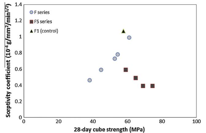
Fig. 6. Sorptivity coefficient against 28-day cube strength.
