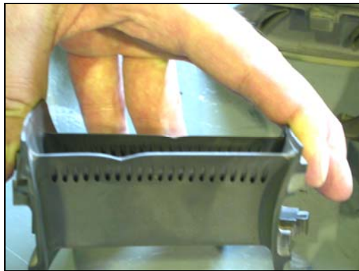
Figure 31 – Damaged HP NGV
