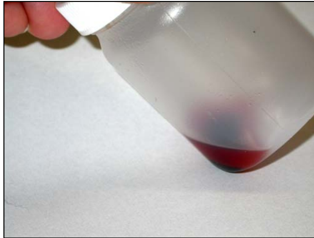
Figure 28 – Liquids Removed From Lobo A2 Coalescing Filter
