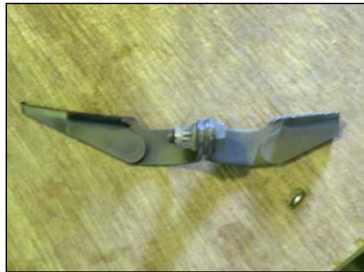
Figure 32- Failed Nozzle Bracket
