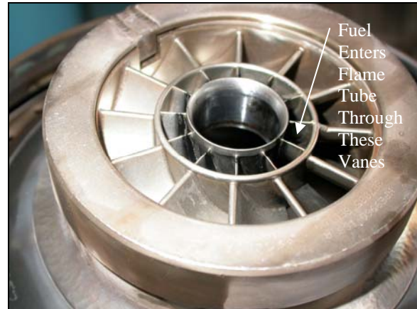
Figure 14 – Swirler Burner Flame Tube
