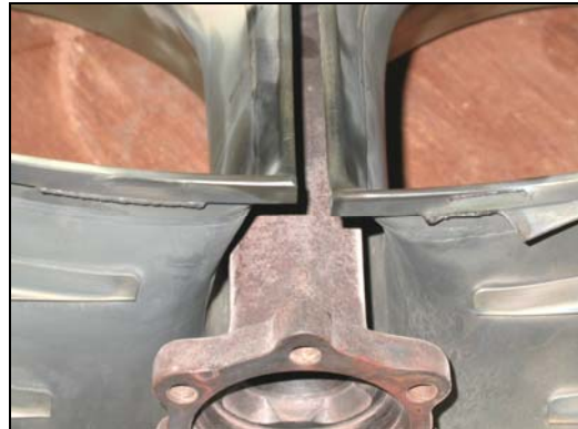
Figure 30 – Failed Nozzle Bracket
