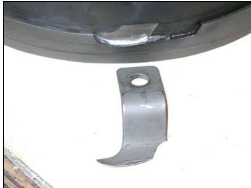
Figure 29 – Failed Chin Strap
