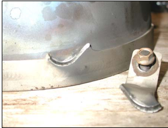
Figure 33 – Failed Chin Strap
