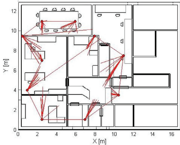
Fig. 5. Positioning error vectors-random sample sps3 with n_{sps} = 10 – WKNN.
