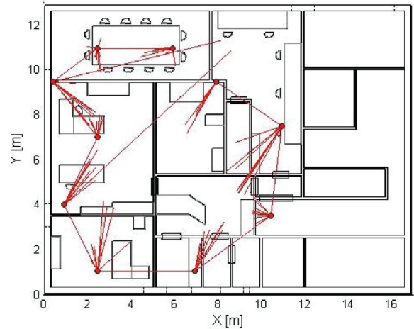
Fig. 6. Positioning error vectors-random sample sps3 with n_{sps} = 10 – MMSE.
