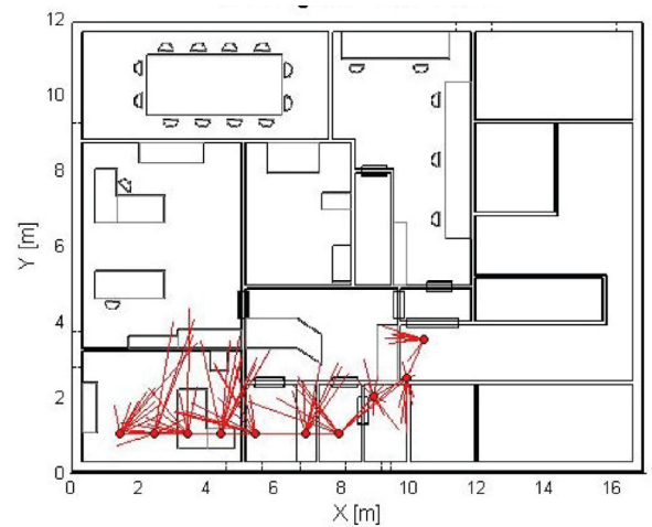
Fig. 3. Positioning error vectors-sample of convenience con5 with n_{con} = 10 - MMSE.
