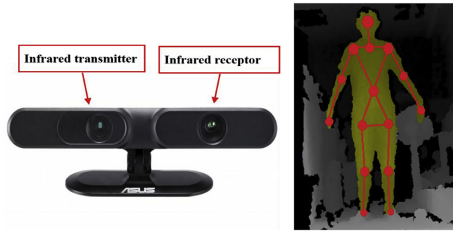
Fig. 3. The ASUS Xtion PRO and human skeleton diagram.
