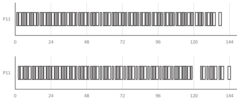
a. Comparison of schedules for the pasteurizer (stage 1) without and with weekend break
