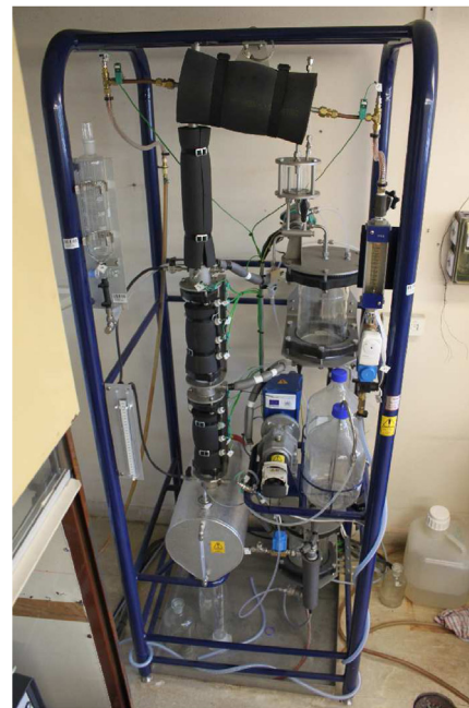
(a) Scheme of the distillation column unit. (b) The UOP3CC laboratory distillation column.
